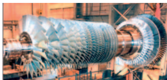
Nonlinear thermomechanical calculation of a combustion turbine compressor: bladed rotor and quarter compressor.
