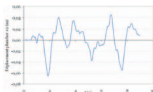
Displacement of the #2 flooring during the seismic
